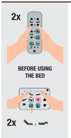
Before you can use the bed, unlock the bed by pushing2x the RESET buttons.
